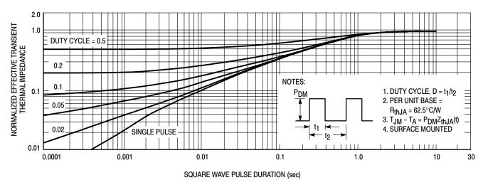
Figure 11. Normalized Thermal Transient Impedance, Junction-to-Ambient
