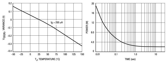
Figure 9. Threshold Voltage
