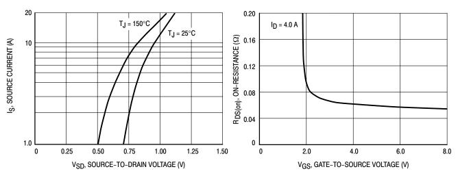
Figure 7. Source-Drain Diode Forward Voltage
